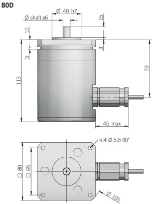
recommended mating shaft tolerance H7 dimensions in mm
